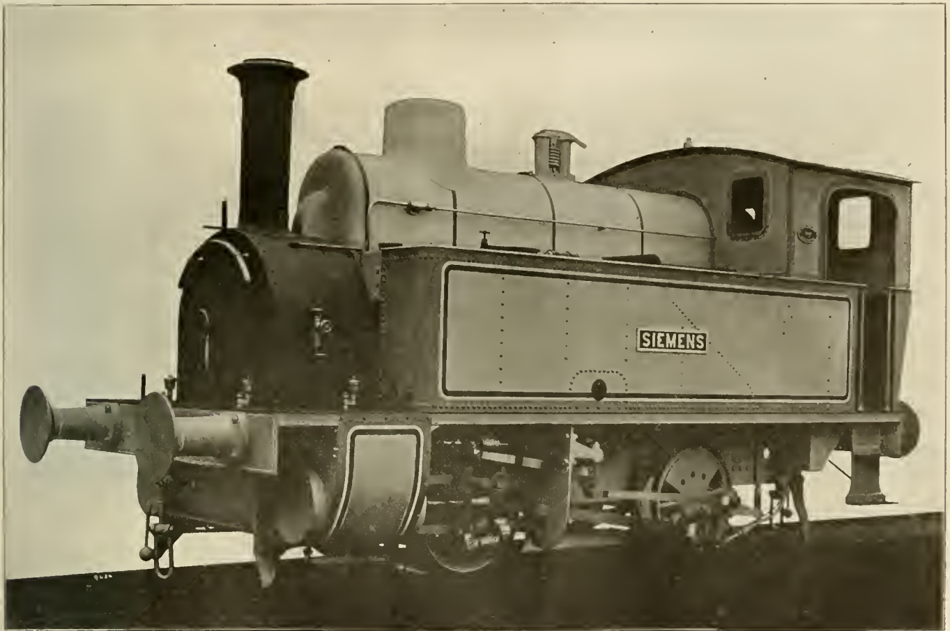
FIG. 1. TANK ENGINE FITTED WITH THE BROTRAN BOILER AND FIRE-BOX.
